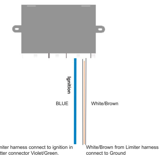
Blue wire from Limiter harness connect to ignition in position 13 of upfitter connector Violet/Green.
