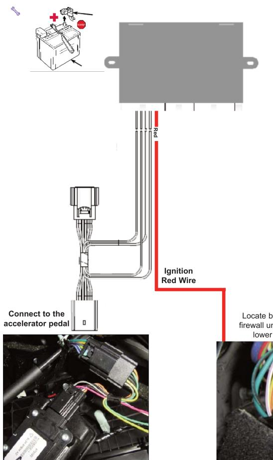
Locate black connector near firewall underneath driver side lower dash panel area
