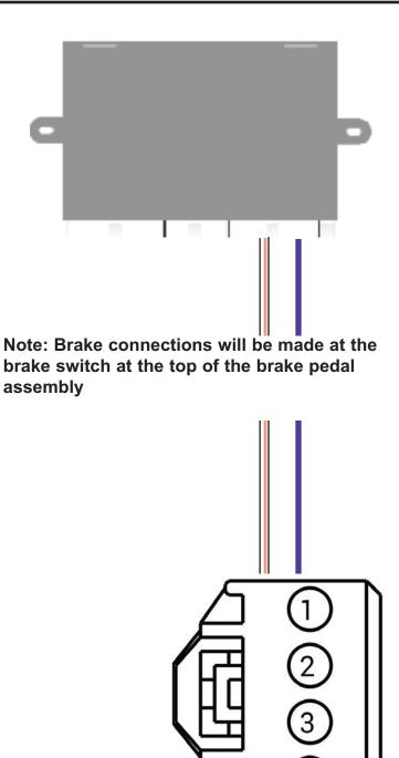
Connect the WHITE/BROWN Rostra negative brake wire to the VIOLET/WHITE wire at the brake switch position 4.
