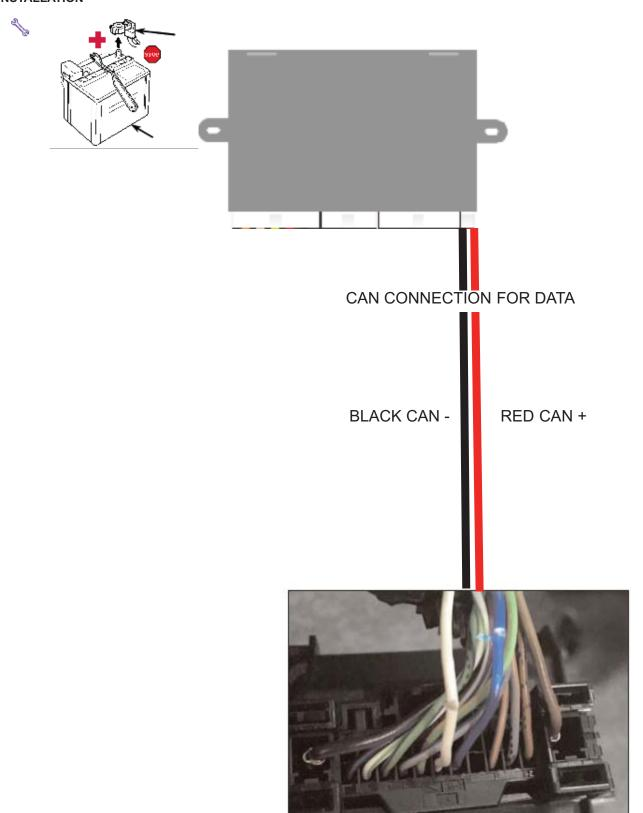
Note: Vehicles Equip. with gateway connector on back of OBD2 solder cruise Red CAN high wire to Blue wire in position 20. Solder Black CAN low wire to White position 19.
