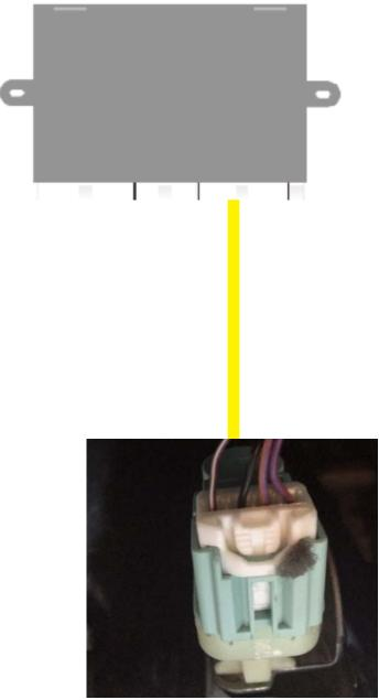
Locate the Brake Switch at top of brake switch assembly. Connect cruise Yellow wire to Violet/White in position 1.
