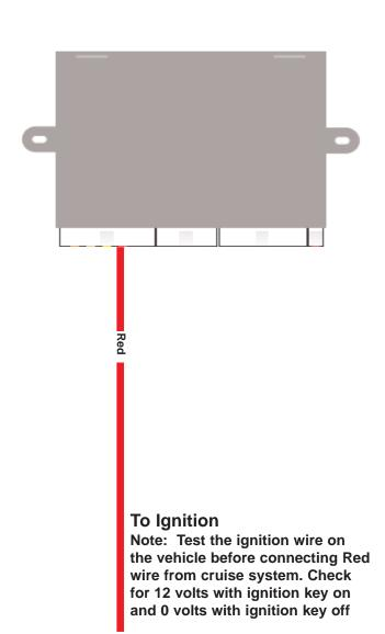
Connect Red ignition wire to Brown/Yellow wire at the ignition switch connector located at left side of steering column.
