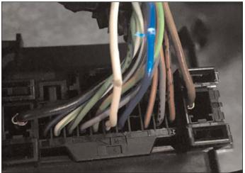
Note: Vehicles Equip. with gateway connector on back of OBD2 solder cruise Red CAN high wire to Blue wire in position 20. Solder Black CAN low wire to White position 19.
