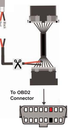
Note: Standard OBD2 Connect Red wire to White/Blue wire in Pin 6 and Connect Black wire to White wire in Pin 14
