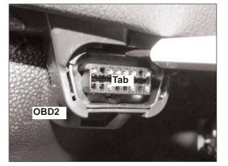
Note: Use a precision tool to press up on the backside of the OBD2 connector housing to release the tab. Push out OBD2 connector toward the back to remove.
