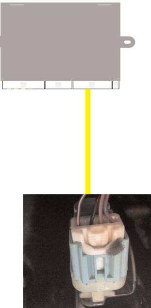
Locate the Brake Switch at top of brake switch assembly. Connect cruise Yellow wire to Violet/White in position 1.
