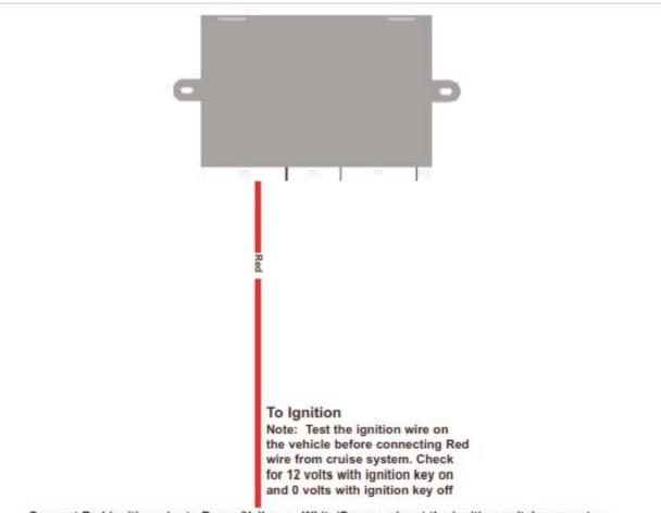
Connect Red ignition wire to Brown/Yellow or White/Orange wire at the ignition switch connector located at left side of steering column.
