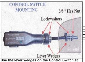
Use the lever wedges on the Control Switch at an angle template to drill a 3/8" or 9.5mm hole
