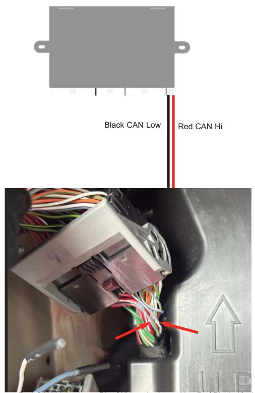
Connect Rostra Red CAN high wire to Blue/White wire in position 7 of Black 48 pin connector behind Drivers Kick panel. Connect Rostra Black CAN low wire to Blue/Yellow wire in position 8 of Black 48 pin connector behind driver kick panel.
