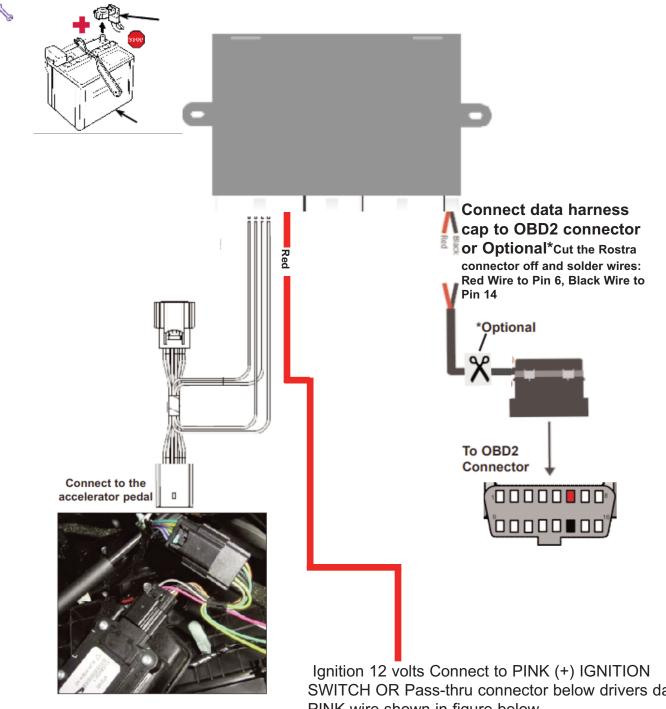
SWITCH OR Pass-thru connector below drivers dash PINK wire shown in figure below.
