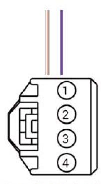
Connect the WHITE/BROWN Rostra negative brake wire to the VIOLET/WHITE wire at the brake switch position 4.
