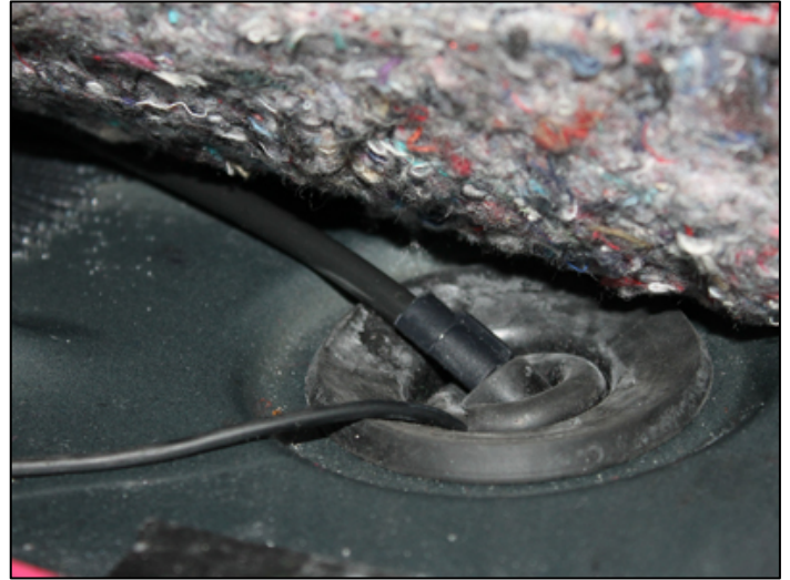
Route harness 250-8579 through the rubber grommet underneath the carpet.
