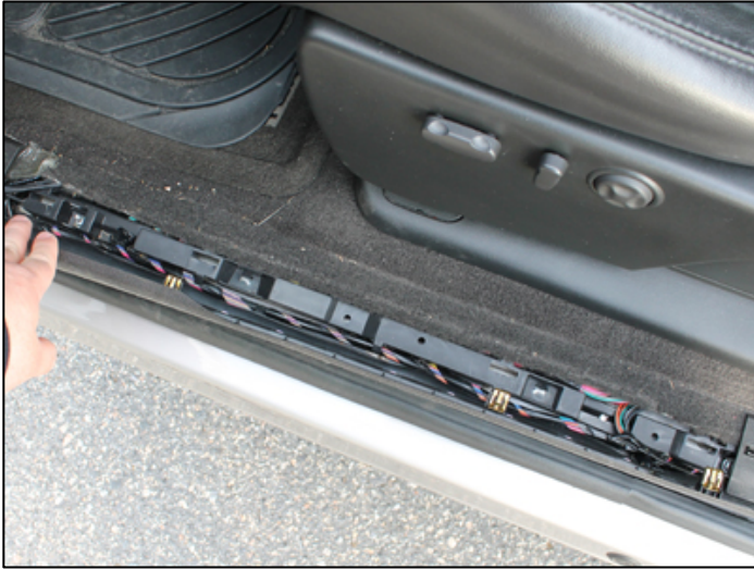
Remove the doorsill trim and gently lift back on the carpet near the driver's seat.
