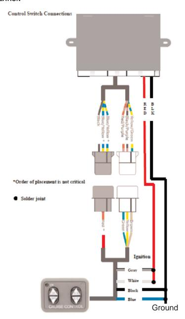
MOUNT DASH CONTORL SWITCH TO THE LEFT OF STEERING COLUMN ON DRIVERS DASH USING TEMPLET PROVIDED IN CONTROL SWITCH PACKAGE/INSTRUCTIONS
