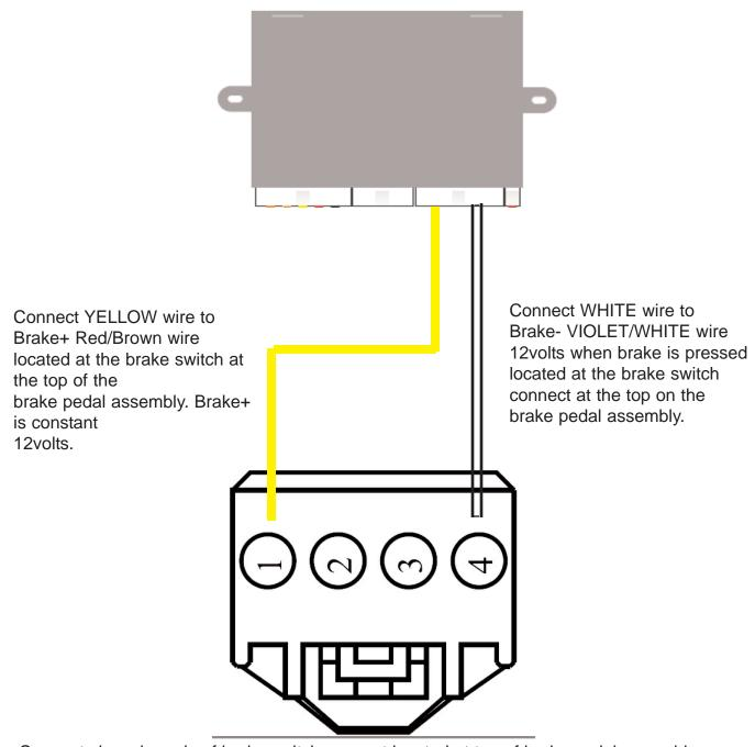
Connect view above is of brake switch connect located at top of brake pedal assembly
