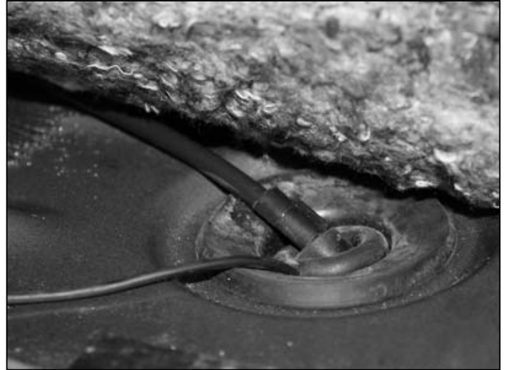
Route harness 250-8656 through the rubber grommet underneath the carpet.
