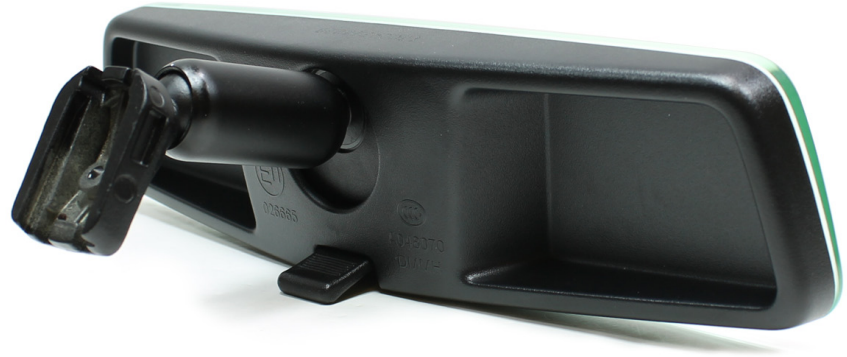
260-8704 Infinity Prismatic. Edge-to-edge mirror glass. Manual dimming.
