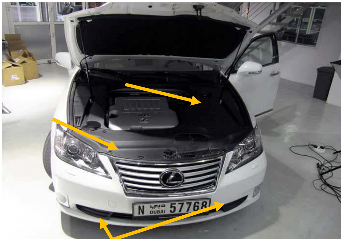
Remove the original bezels, radiator cover and the under hood fuse box cover.
