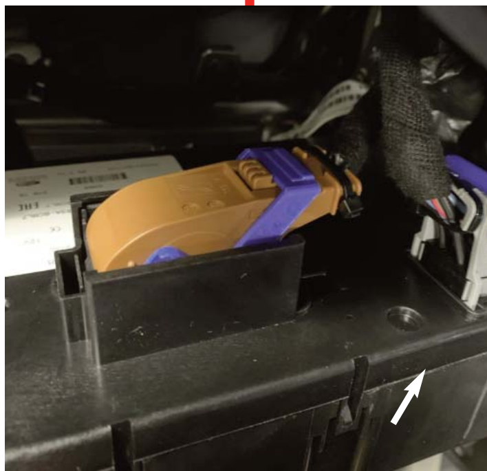
BCM Brown connector in rear of BCM/fuse box 60 pin plug. Connect Rostra Red ignition wire to DK. Blue wire in position 12
