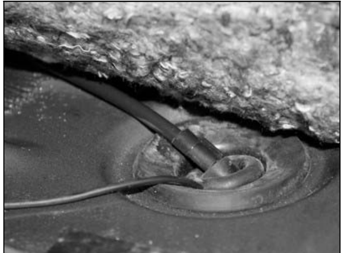
Route harness 250-8550 through the grommet in the floor board on the driver side of the truck.
