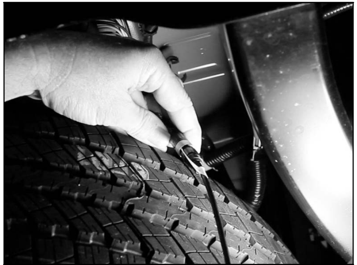
Feed the camera harness into the opening of the truck bed and connect to 30' extension harness 250-8550.
