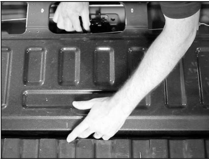
Wrap the camera harness with convoluted tubing and route it to the bottom tailgate opening.
