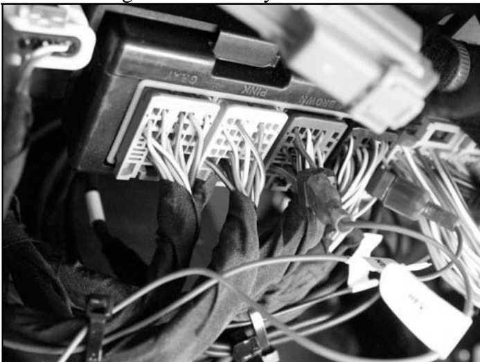
Locate the BCM connectors behind the driver-side dashboard knee panel.
