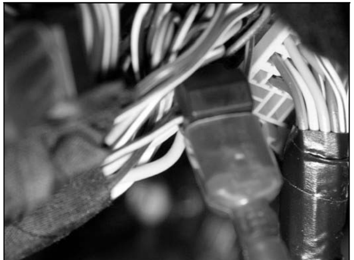
From harness 250-8505, connect the black w/white stripe wire to the green w/violet wire of the fourth from left BCM plug using the included t-taps.
